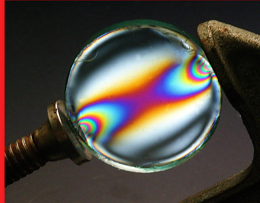
Stress patterns in a glass disk caused by pressure of jaws of a C-clamp: Photograph by Andrew Davidhazy (2009)
